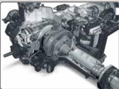
**Full Powershift transmission,** provides seamless smooth shifting from zero to 40 or 50 kph. Creeper gears offer an additional 10 speeds from 225m/h to 1.6 kph @ 2,200 rpm.
