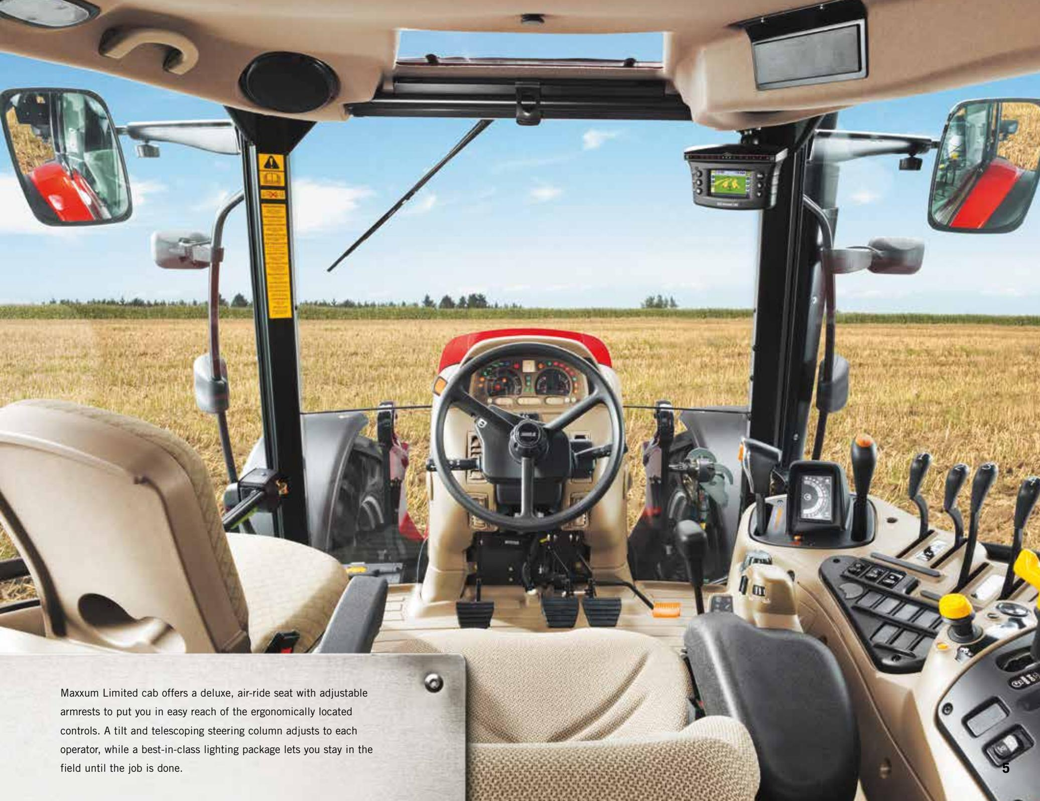
Maxxum Limited cab offers a deluxe, air-ride seat with adjustable armrests to put you in easy reach of the ergonomically located controls. A tilt and telescoping steering column adjusts to each operator, while a best-in-class lighting package lets you stay in the field until the job is done.
