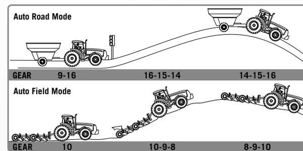
**Autoshift option for road and field gears** on Maxxum Limited models provides automatic shifting based on load.
