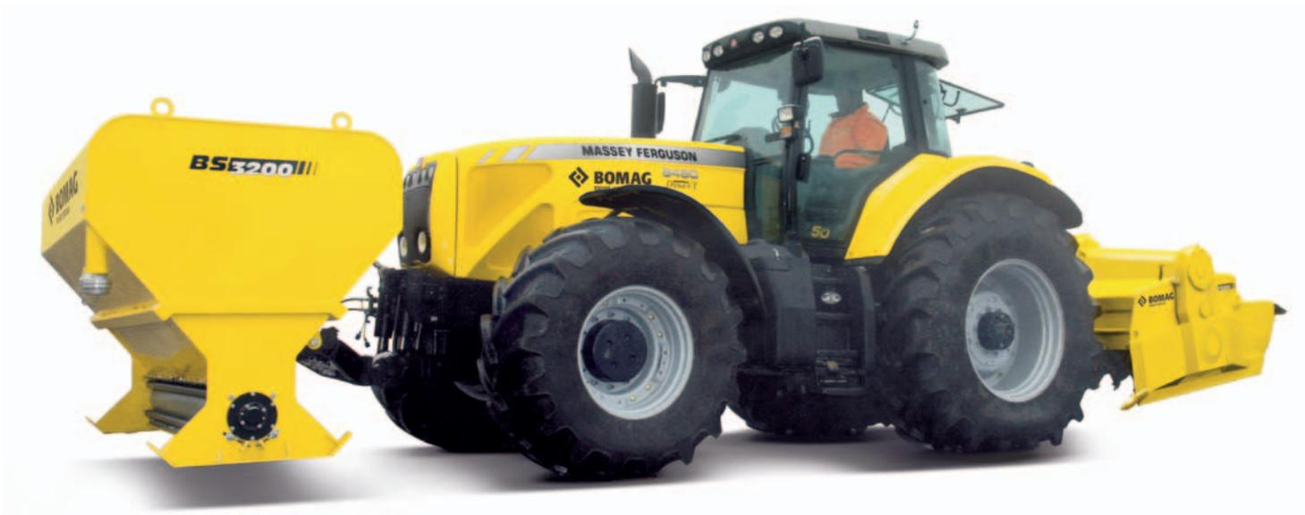
With a payload of 3,200 kg the BOMAG spreader is designed for small and medium-sized work and areas with difficult access. The 2,500 millimetre wide rotor ensures uniform spread of binder. The metering system is driven by the carrier unit's hydraulics. The hydraulic motor for the rotor can be progressively adjusted by an oil flow control valve on the tractor.
