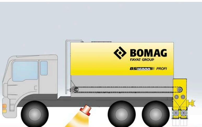
Feed monitoring with filling level sensor.
