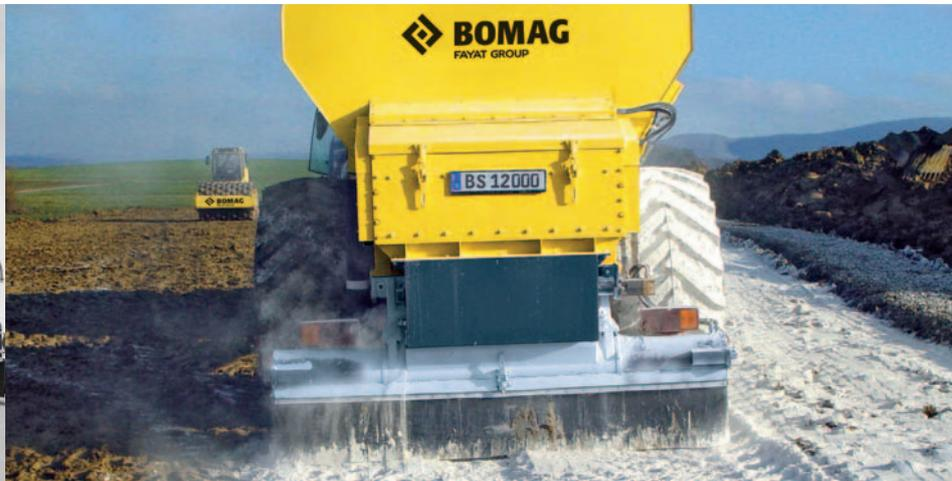
Soil stabilisation and cold recycling have long been accepted as economical and environmentally friendly methods of converting weak soils into stable foundations, and for renewing road bases while saving resources. The addition of hydraulic binders has been proven especially on difficult materials.
