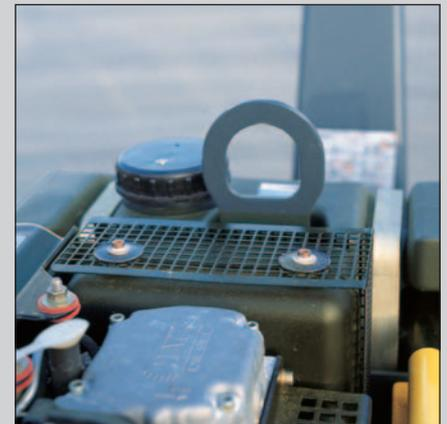
Central lifting eye and lateral tie-down lugs for fast and safe transportation.
