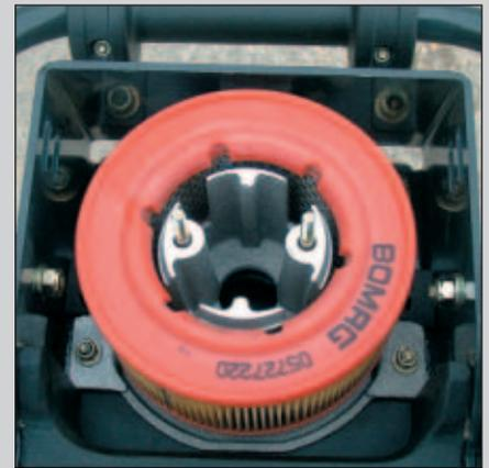
Near-zero maintenance expenditure with self-cleaning air filter housing and large air filter element.
