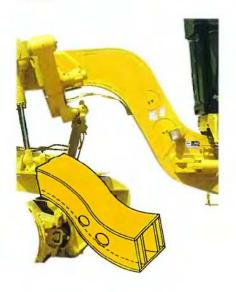
Circle drive slip clutch – protects circle shoes and teeth from damage. Should a large rotational force be placed against the blade (as when striking a buried rock) the clutch will slip and the impact load placed against frame will also be absorbed.
