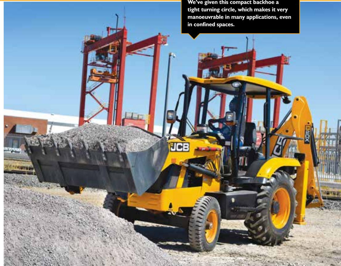
5 Our multi-position rear excavator minimises repositioning; it also means the 2DX can easily dig parallel to walls or in an off-centre position for better visibility to the trench. The digger arm can be quickly and easily positioned and hydraulically locked across the rear frame without the driver leaving the seat.
