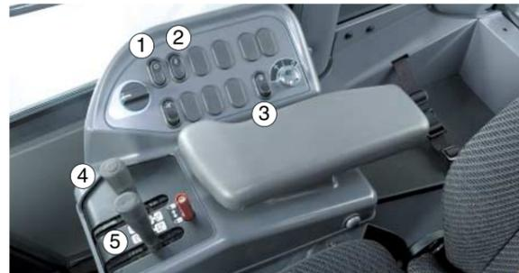
1:Cut-off ON/OFF switch 2:Cut off adjustment switch
