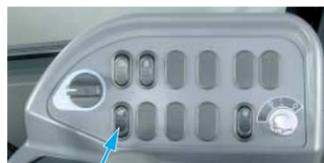
Dual mode engine power selection switch
