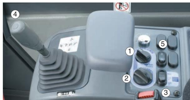
1:Speed range selector switch 2:Variable shift switch
