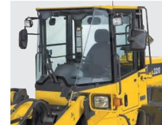
provides maximum space for the operator. The front mounted air conditioner was introduced to increase seat reclining and backward slide adjustment.
