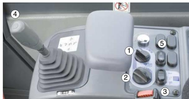
1:Speed range selector switch 2:Variable shift switch
