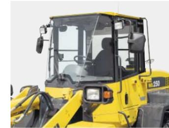
provides maximum space for the operator. The front mounted air conditioner was introduced to increase seat reclining and backward slide adjustment.
