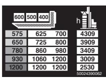
Load carrying vs. lift height relationship shown by colour code on the mast (Option).
