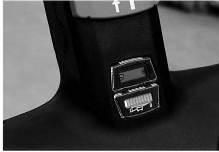
Clear display of battery condition and operating hours
