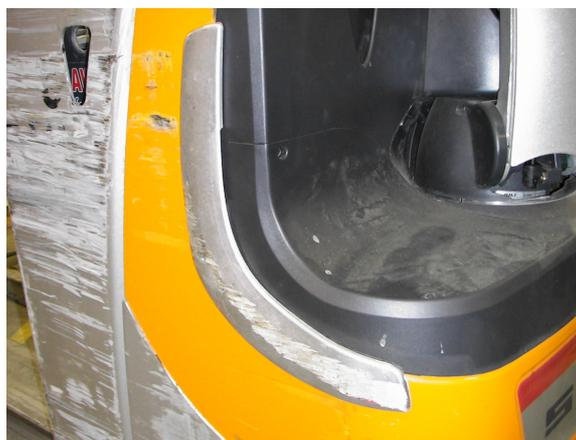
We have received several complaints about damaged or torn off motor covers on EXU – trucks and we have decided to set up in series a metallic protection.
