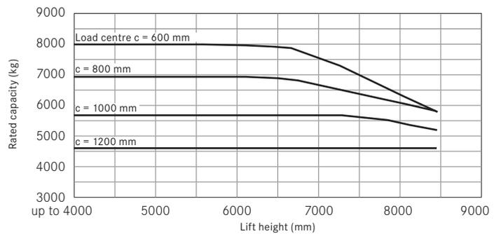
Different tyres, other masts, additional equipment etc. could give different figures.
