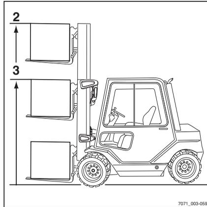
**Malfunction during a lifting operation****Incorrect extension sequence****⚠ DANGER****Risk of accident!**
