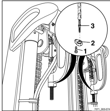
**Setting the load chains triplex mast**
