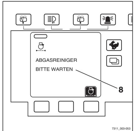
Faults in the regeneration process are shown by the message **ABGASREINIGER (EXH. GAS PURIFIER)** (9). The faults must be corrected by the service centre.
