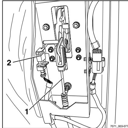
**Lubricating the parking brake lever bearing and ratchet**
