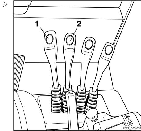
**Lifting system, multi-lever operation** ▷
