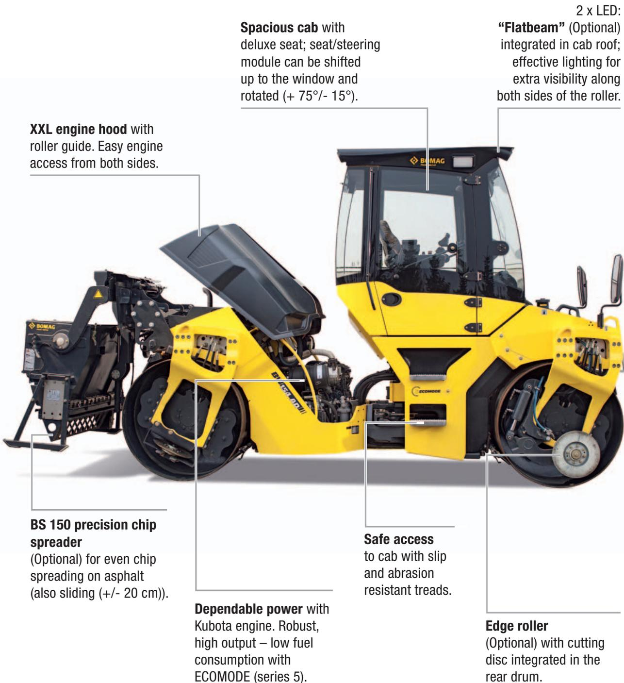
**Spacious cab** with deluxe seat; seat/steering module can be shifted up to the window and rotated (+ 75°/- 15°).
