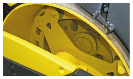
Direct drum drive with vibrating travel speeds of 4.5 mph available. Individually serviceable isolators without drum removal.
