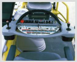
Operator's control panel is fully adjustable to either seating position. Simplified controls make operation easy to novice, as well as experienced operators. Display panel provides all necessary, as well as critical information for proper machine operation and professional results.
