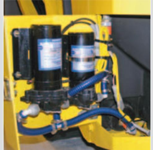
Dual water spray pumps, providing back-up provision.
