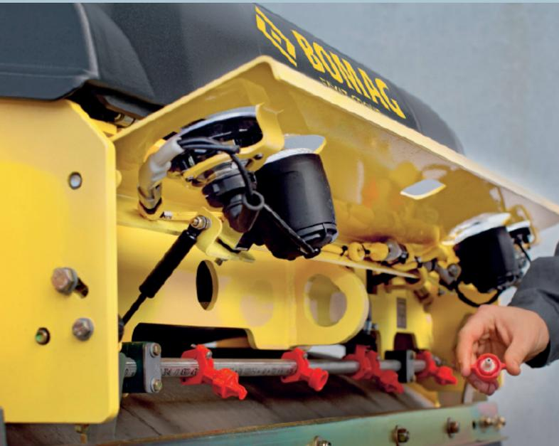
Robust and easy to maintain: the wind-protected sprinkler system behind the engine hood and tailgate.
