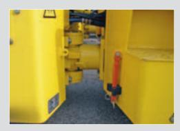
Bolt-on, maintenance free, center-joint with standard crab steer off-set, provides long life and ease of repair.
