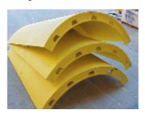
Smooth Shell Kit for padfoot drum equipped rollers.
