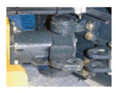
Bolt-on oscillating, articulation joint for long life and servicing ease
