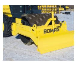
BW145PDH-40 Padfoot model for cohesive material. Also available with optional leveling blade.
