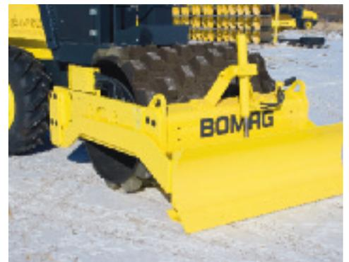
BW145PDH-40 Padfoot model for cohesive material. Also available with optional leveling blade.
