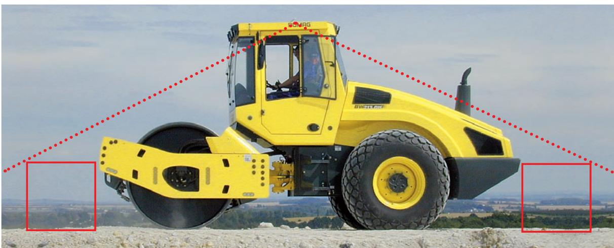
BOMAG single drum rollers meet the 1x1m rule.
