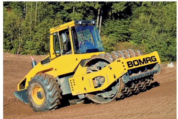
Power and versatility on landfill site construction: BW 213 DH with pad foot shell and tractor tyres.
