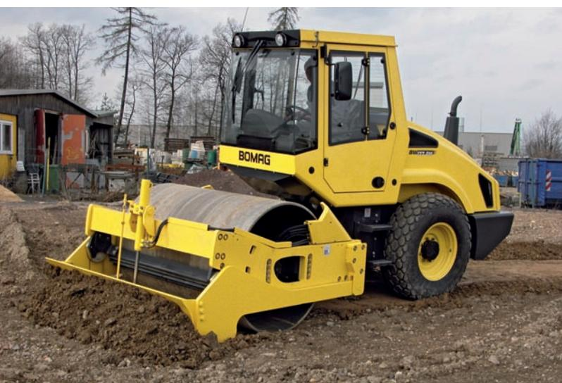
Spread and compact at the same time: Single drum roller with dozer blade, in this case a BW 177 DH-4.
