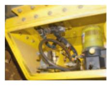
Automatic Central Lube System reduces maintenance time
