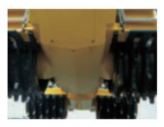
The sealed tub design protects drive components
