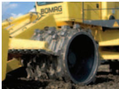
Scrapers positioned at both the front and rear of the drum to ensure a clean drum surface for maximum tooth penetration
