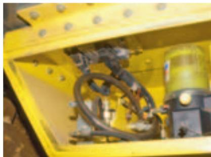
Automatic Central Lube System reduces maintenance time
