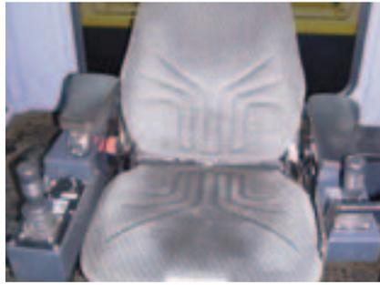
Air Ride Heated Seat and ergonomic joystick controls reduces operator fatigue
