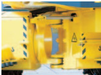
Oscillating, articulated center joint assures that all 4 wheels have ground contact for optimum compaction, gradeability and safety
