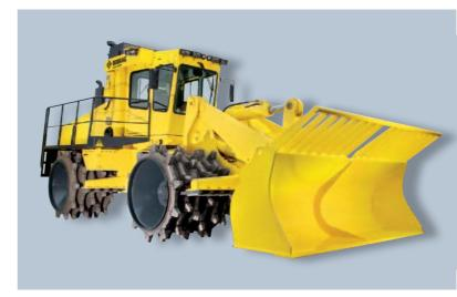
RS version with lifting gear and bucket.
