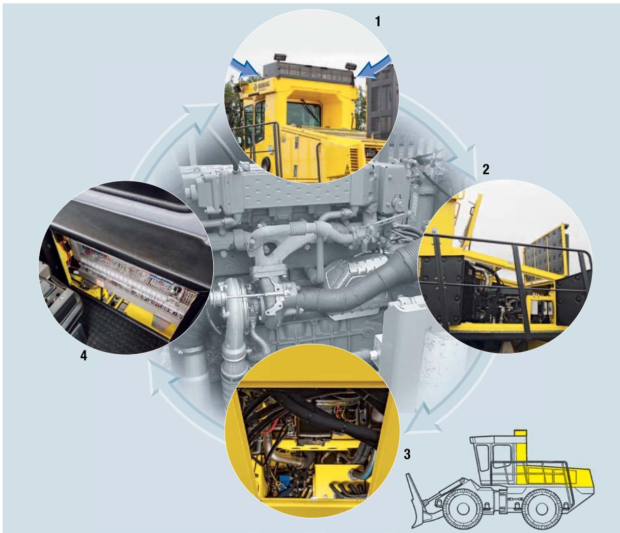
**1 High level suction** for cooling and combustion air with **minimum dust levels.**
