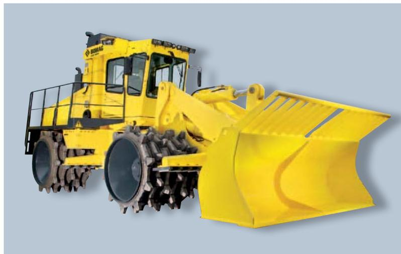
RS version with lifting gear and bucket.
