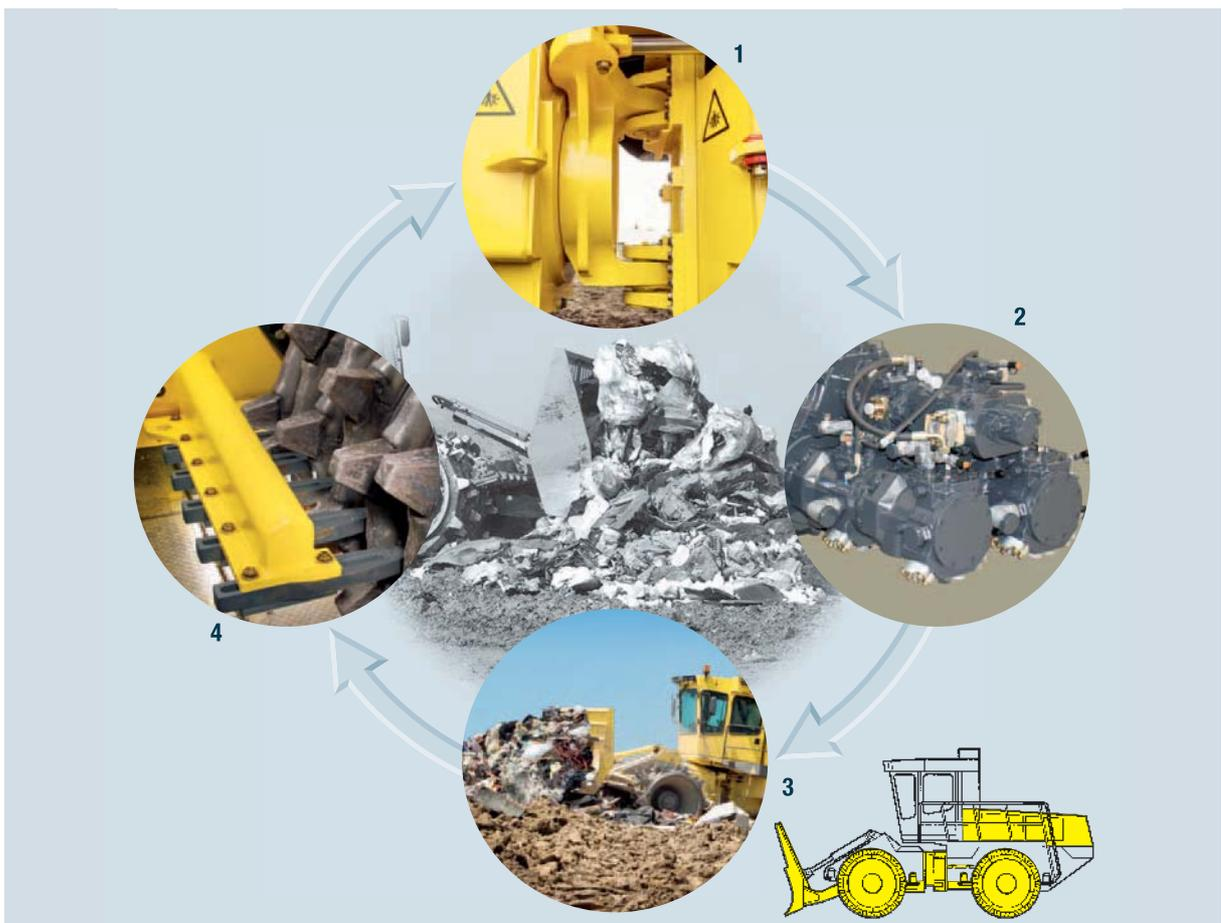
**1 High traction** with the oscillating articulated joint (continuous ground contact).
