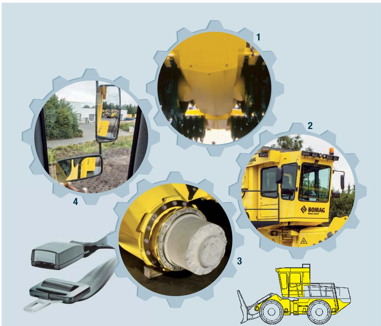
**1** Frame with enclosed sections for best possible protection of all components and no ingress of material; no danger of ignition on hot components.
