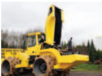
Efficient Component Access with a Vertically Opening Hood
