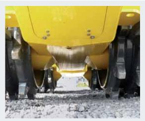
Frame with enclosed sections for the best protection of all components; no ingress of material and nothing to ignite on hot components.
