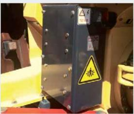
Ground level access to the battery box and main switch.
