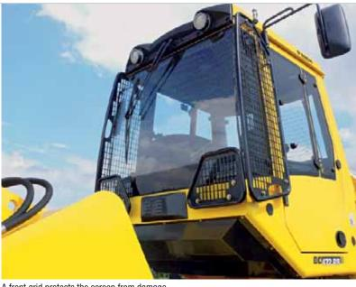
A front grid protects the screen from damage.
