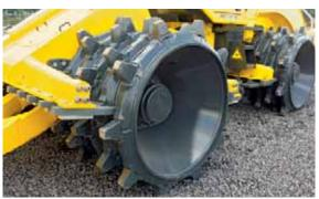
Welded wheel sections with inner taper on both sides for optimum stability
