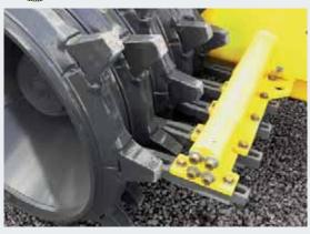
Clean wheels with two-way acting scrapers (and for optimum compaction).
