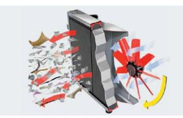
$\dots$  dust and coarse particles are blown out from the radiator grid and air grilles.
