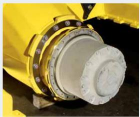
Two independent braking systems (hydrostatics for the service brake, multiple discs for the parking brake).
