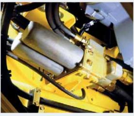
Electronically monitored filter system for cost-effective operations.
