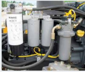
Three stage fuel filters ensure the long life of the injection system.
