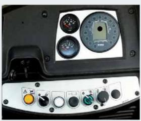
All important features are arranged directly in the field of vision ensuring the operator is always kept up-to-date with his machine.
