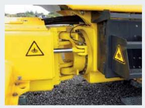
Optimum traction is provided by the oscillating articulated joint (continuous ground contact).
