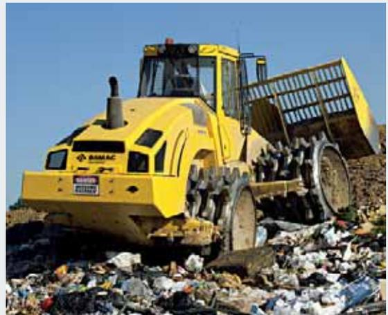
Optimal compaction due to the oscillating joint which generates the necessary load distribution to all wheels.
