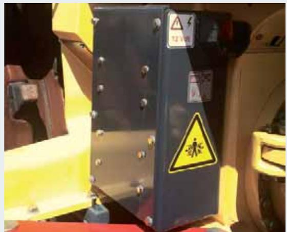
Ground level access to the battery box and main switch.
