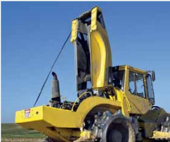
Large maintenance openings for easy access to all drive components.
