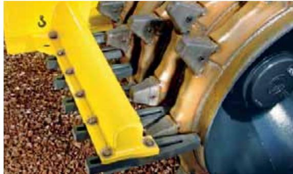
Adjustable scrapers give uninterrupted operation.
