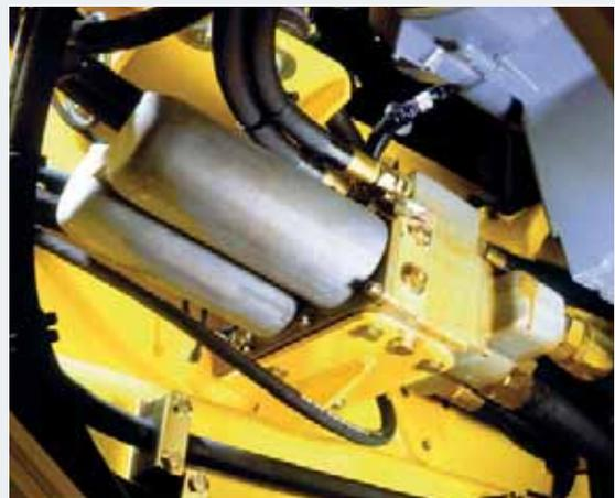
Electronically monitored filter system for cost-effective operations.
