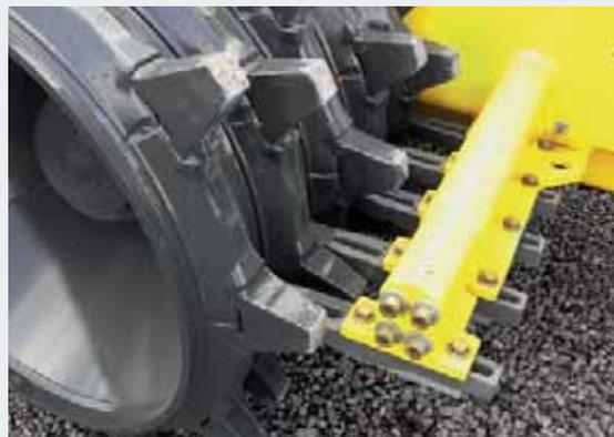
Clean wheels with two-way acting scrapers (and for optimum compaction).
