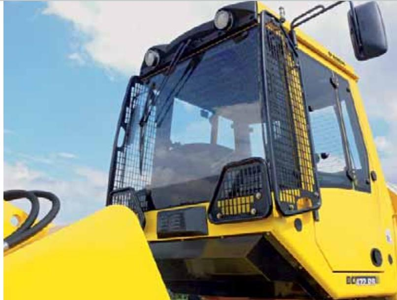
A front grid protects the screen from damage.
