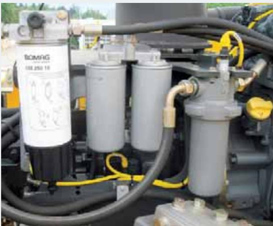
Three stage fuel filters ensure the long life of the injection system.
