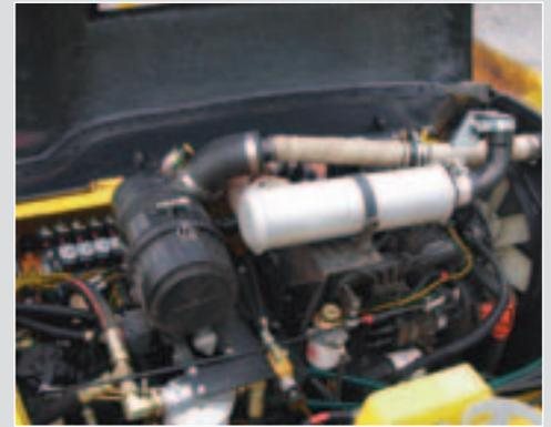
The 60 horse power Cummins diesel engine is protected by a high water temperature, low oil pressure shut down system.
