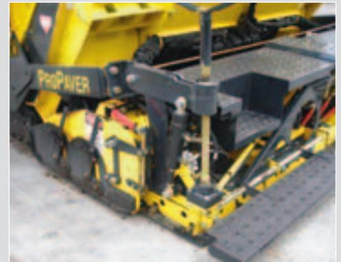
Power depth adjustment controls mat thickness.
