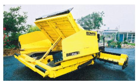
The hopper of the BOMAG BF814 / BF815 can be raised over 6' high, allowing for easy maintenance access to the undercarriage.
