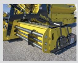
The screed extensions of the BF814 / BF815 have been designed to give the operator exceptional control of the material, as well as a uniform, fully screeded mat.
