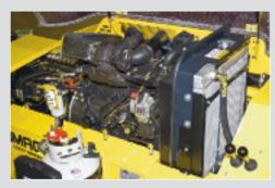
The BOMAG BF814 / BF815 water cooled, 85 Hp diesel engine supplies the power to the hydrostatic drive and pumps.
