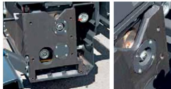
All mechanical extensions are interchangeable between the two screeds, meaning the utilization of paver fleets can be highly optimized.
