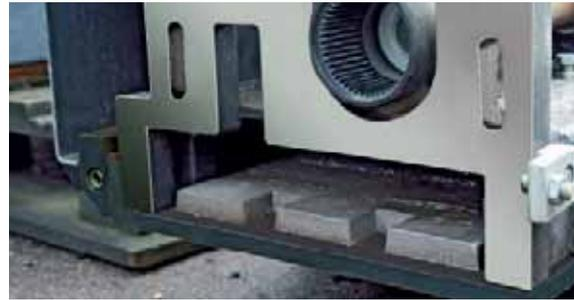
The **powerful heating generator** with a continuous output of 30 kW and the energy efficient aluminium plates cut heating times to 30 minutes even with mechanical extensions.
