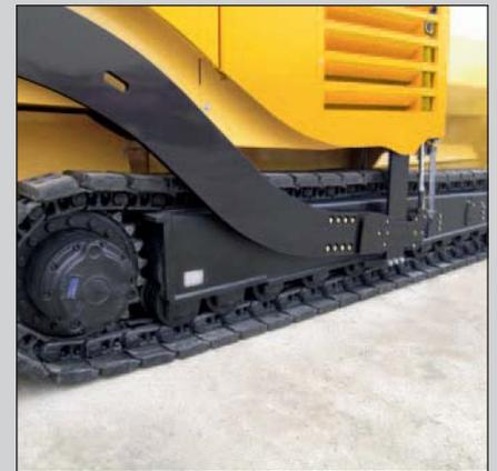
Maximum stability and traction power: BF691C with 3.1 m crawler track.
