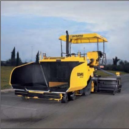
Unobstructed view to front wheels, screed board and hopper with the adjustable SideView System®.
