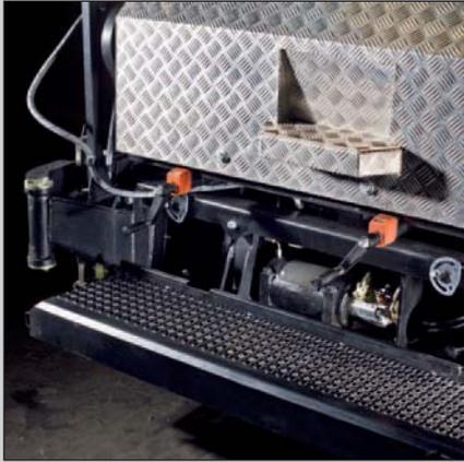
Low step heights, continuous foot board and folding crank handles for easy access.
