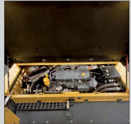
The engine compartment is accessible from four sides.
