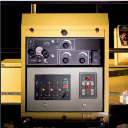
Automatic screed board relief L.C.S.®, screed heating and tamper/vibration setting.
