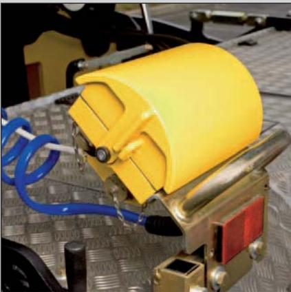
Lockable metal lateral control stands, individually exchangeable controls.
