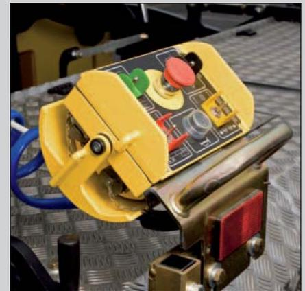
Lateral operator station with exchangeable controls.
