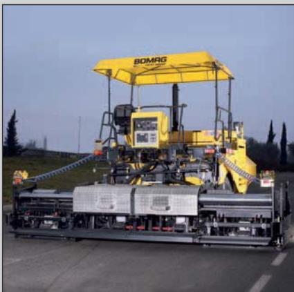
HSE screed board with electric heating and 2.55 m basic width Here extended to 5 m. Optional gas heating.
