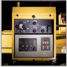
Automatic screed board relief L.C.S<sup>®</sup>, screed heating and tamper/vibration setting.
