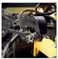
Accurate centring of the screed board with push/pull rod prevents lateral floating.
