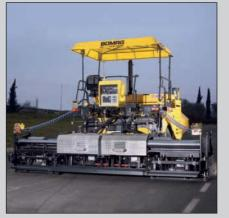
HSE screed board with electric heating and 2.55 m basic width Here extended to 5 m. Optional gas heating.
