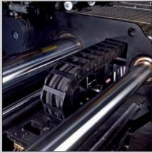
Heavy duty guides prevent bending and torsion of screed board.
