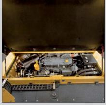
The engine compartment is accessible from four sides.
