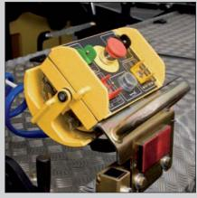
Lateral operator station with exchangeable controls.
