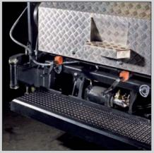
Low step heights, continuous foot board and folding crank handles for easy acess.
