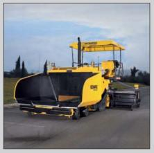
Unobstructed view to front wheels, screed board and hopper with the adjustable SideView System<sup>®</sup>.
