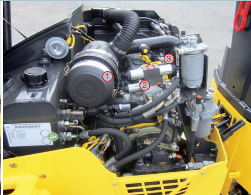
Easy checks: Air (1), oil (2), water (3) – fast access: time saving.
