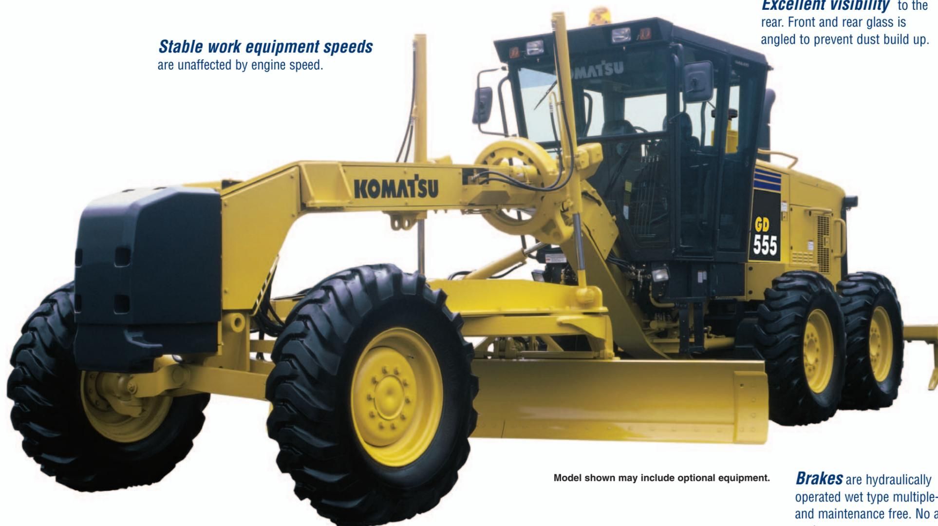
High performance engine **Komatsu SAA6D102E turbocharged and air to air aftercooled** diesel provides 119 kW **160 HP** for demanding applications.
