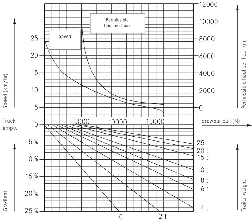
The Speed/Draw Bar Pull performance of the tractor can be programmed between the two limits shown to suit the application. The permissible haul per hour is the total distance travelled, including the return journey and any downhill gradients. It is recommended that braked trailers are used for trailer loads exceeding 9 tonnes and for all trailer loads if gradients are involved.
