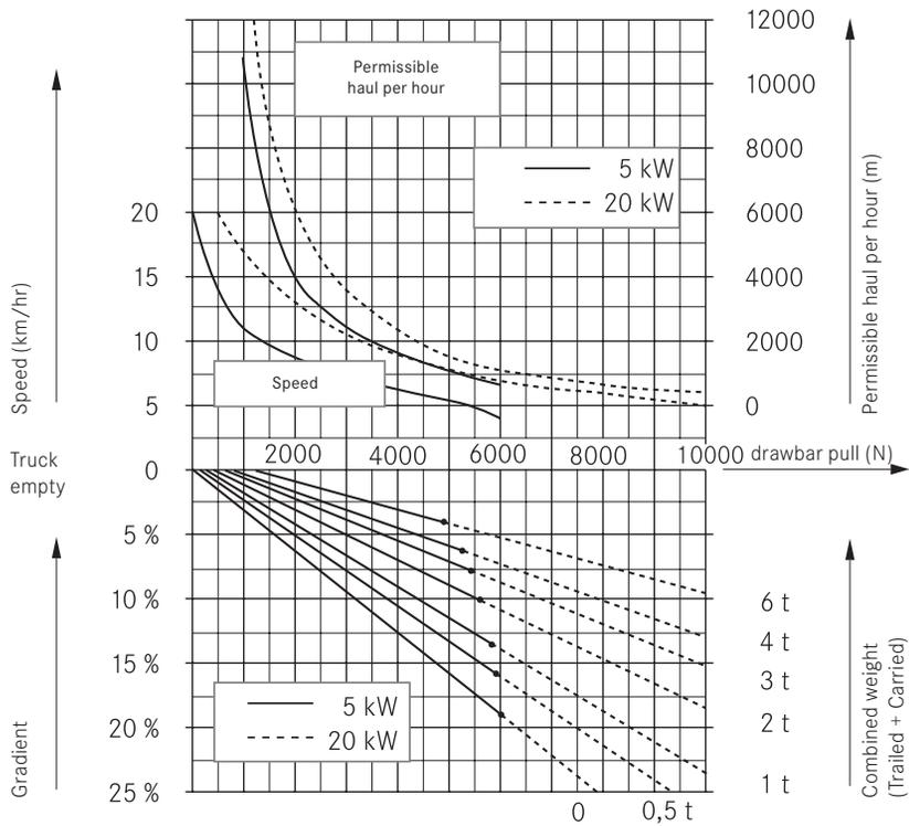
The permissible haul per hour is the total distance travelled, including the return journey and any downhill gradients. It is recommended that braked trailers are used for all trailer loads if gradients are involved.
