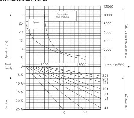
The Speed/Draw Bar Pull performance of the tractor can be programmed between the two limits shown to suit the application. The permissible haul per hour is the total distance travelled, including the return journey and any downhill gradients. It is recommended that braked trailers are used for trailer loads exceeding 9 tonnes and for all trailer loads if gradients are involved.
