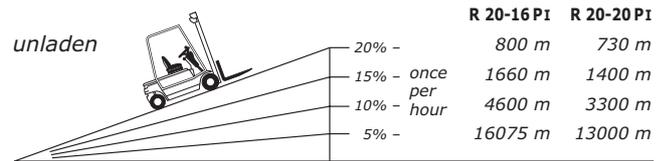
**Example** (with 2000 kg load): 9% gradient, 10 m distance. This gradient is negotiable 128 times per hour.
