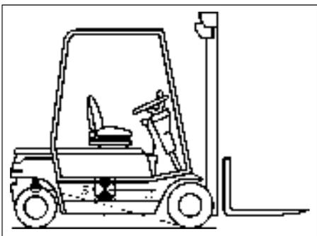
Stability is achieved by virtue of the high position of the steer axle articulation point. This means that the centrifugal force has less effect because of the short length of its lever arm from the tipping line.
