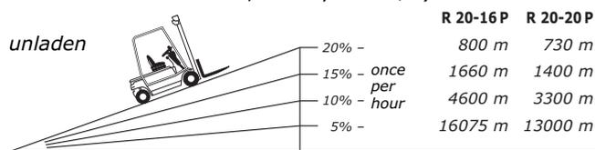
**Example** (with 2000 kg load): 9% gradient, 10 m distance. This gradient is negotiable 128 times per hour.
