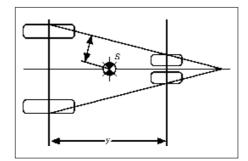
Due to a long wheel-base and twin rear wheels, the tipping lines are spread widely apart and thus are a long way from the truck's centre of gravity. The greater this distance, the higher the stability.
