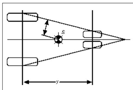
Due to a long wheel-base and twin rear wheels, the tipping lines are spread widely apart and thus are a long way from the truck's centre of gravity. The greater this distance, the higher the stability.
