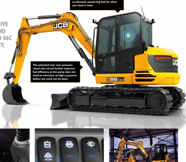
The load-sensing hydraulics on JCB's 8-tonne excavators only consume power
