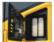
External air conditioner filter
