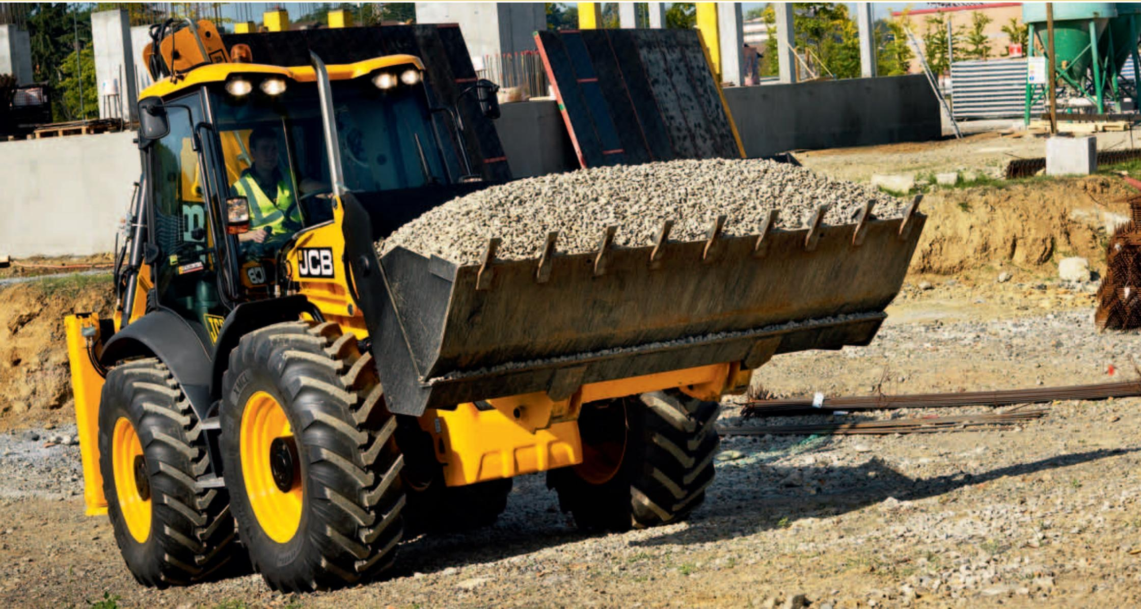
Engine Power: 88kW (118hp) Backhoe Dig Depth: 6.51 metres (21ft 4in) Loader Capacity: 1.3m<sup>3</sup> (1.70yd<sup>3</sup>)
