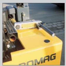
Safety crank handle always at the machine (accept BW 75 H).
