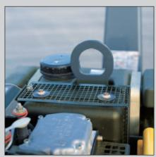
Central lifting eye and lateral tie-down lugs for fast and safe transportation.
