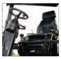
BW 141AD-4 / BW 151AD-4 Operator's platform with sliding/swiveling seating position
