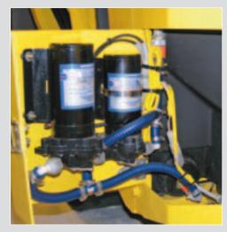
Dual water spray pumps, providing back-up provision.
