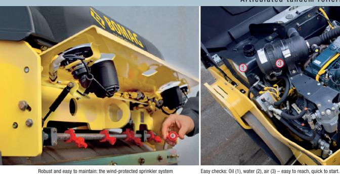
Robust and easy to maintain: the wind-protected sprinkler system behind the engine hood and tailgate.
